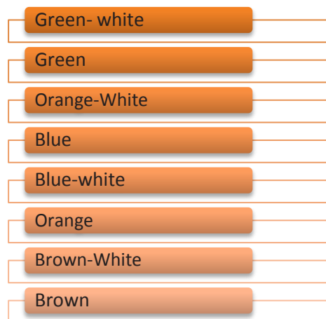
Fig. 3.4.5: Color code for crimping RJ45 crossover cable
