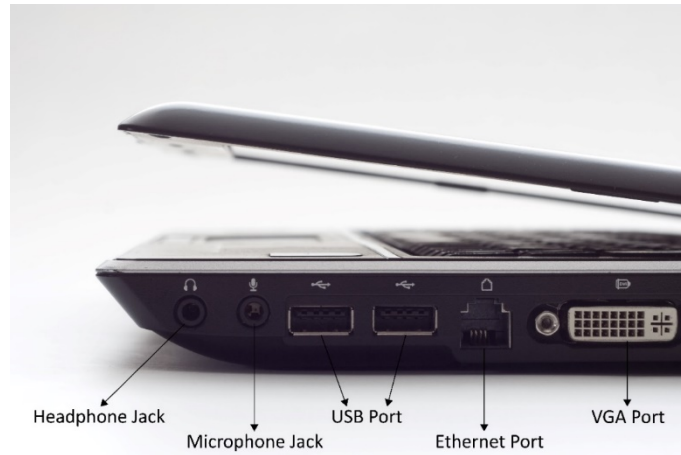
Fig. 4.1.7: Different connection ports in a laptop computer
